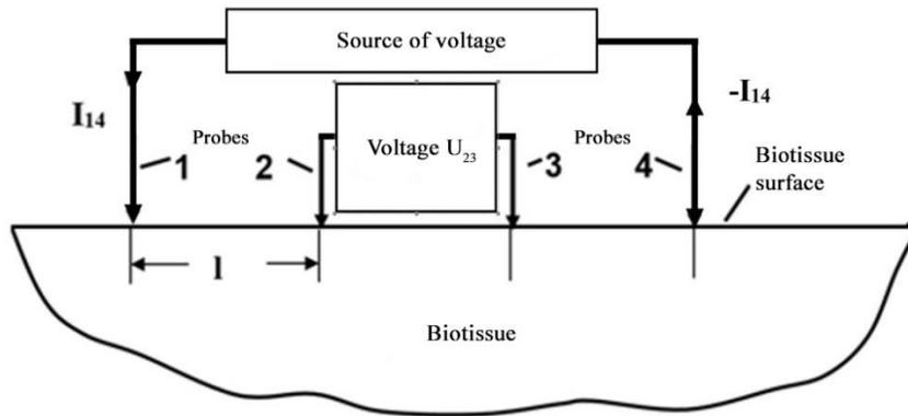
Figure 6. Measurement scheme with four probe methods.
