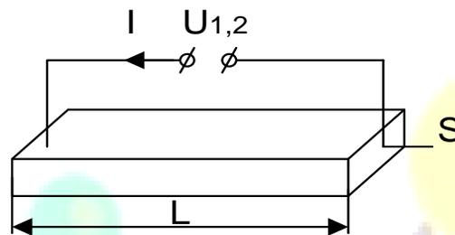
Figure 5. Two-probe method detection scheme.
