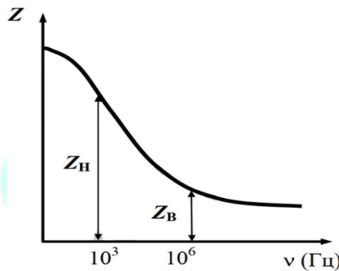
**Figure 4. Dependence of tissue impedance on current frequency and determination of values included in the formula (4)**
