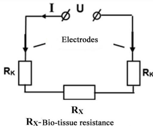
Figure 7. Equivalent circuit of the two-electrode method.
