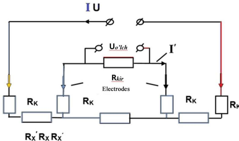
Figure 8. Equivalent scheme of the four-electrode method
